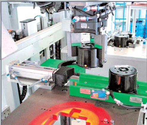
Handling unit with gripper system in an assembly unit for ABS components.
